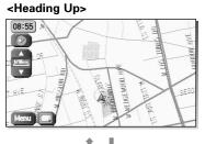
Selecting s rotates the map to so that direction you are heading is always shown as upwards on the screen (the red arrow indicates North):
